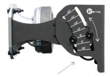
Adjust the required vertical radiation angle according to the height of the installation. · Four screws on both sides must be fastened according to the scale.
